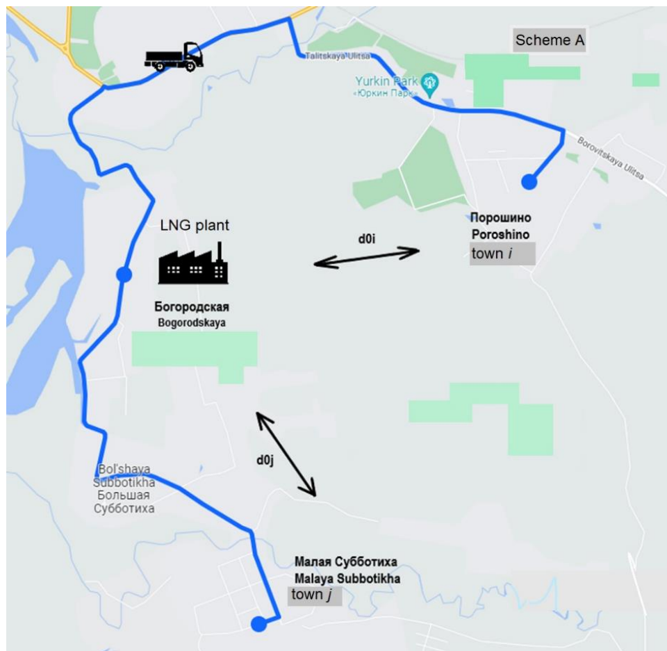
Figure 1. Gas delivery option according to the dead-end scheme A (authors drawing)
