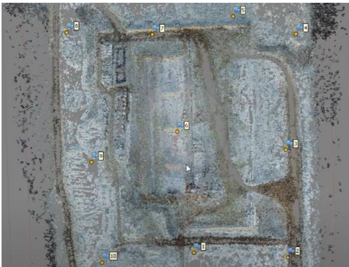
Рисунок 6. Опорные точки на площадке работы дрона ( https://banumukhtar.com/news/banumukhtar-joins-hands-with-turkish-counterparts-for-construction-of-hayat-kimya-green-field-project-at-fiedmc/ )
